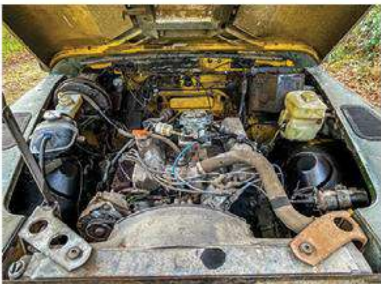
Engine bay as found, with Weber twin-choke carb and homemade manifold
