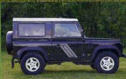
CE QUE VOUS AVEZ SOUS LES YEUX EST L'UN DES LAND LES PLUS RARES AU MONDE. PLUS EXACTEMENT, CE N'EST PAS VÉRITABLEMENT UN DEFENDER TEL QU'ON LE CONNAÎT, MAIS UN PROTOTYPE. DÉVELOPPÉ EN 1996 AFIN D'ÉVALUER LES POSSIBILITÉS OFFERTES PAR UNE STRUCTURE MONOCOQUE ENTIÈREMENT EN ALU, IL NE POSSÈDE PAS DE CHÂSSIS TRADITIONNEL. SI PLUSIEURS EXEMPLAIRES ONT ÉTÉ PRODUITS, IL EST LE SEUL RESCAPÉ. **Par Jérôme André**
