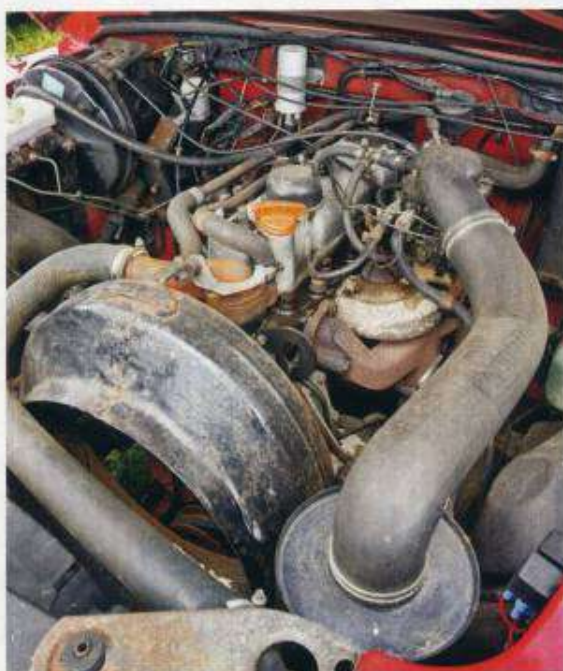
Fitted with the twin choke Weber, engine is good for 74bhp
