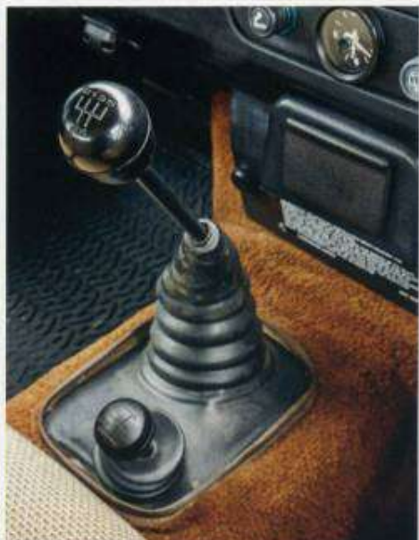
Standard five-speed LT77 gearbox, knob is later type
