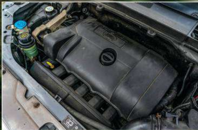
Volvo's transverse-mounted straight-six is a snug fit
