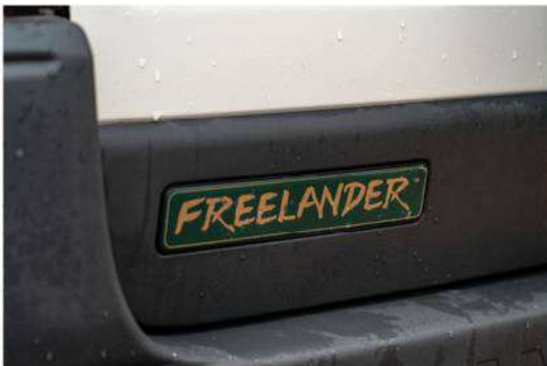
Moulding recess for badge was designed for planned Highlander name, which turned out to be owned by Volvo. Second choice name had to be the same length!
