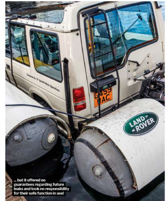
Airbags were repaired by the original manufacturer and tested to 4psi...
