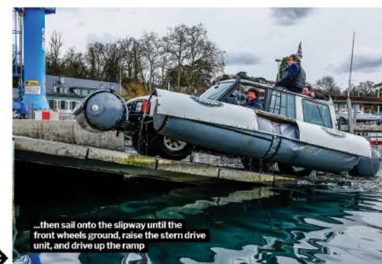
Simply drive down the slipway until the vehicle is floating, lower the stern drive unit, and off you go...
