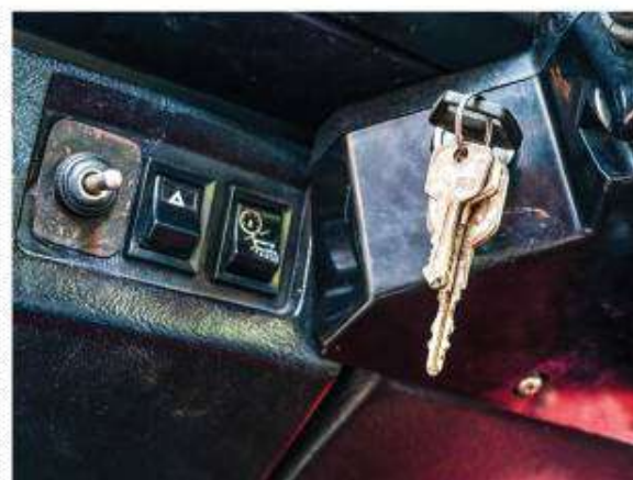
Smooth plastic around column and switches fitted direct to lower heater duct are non-production items. Keys are original
