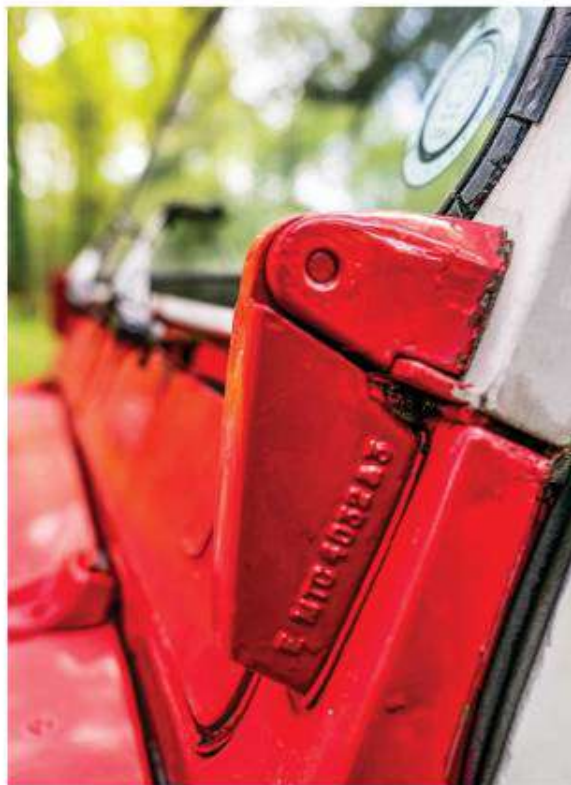
Plenty of special pre-production features: both windscreen hinges have casting numbers on them
