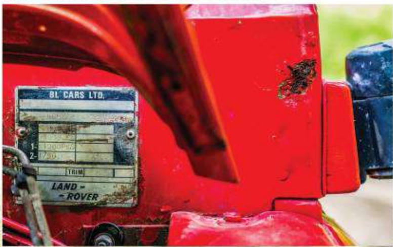
VIN plate on pre-pro is mounted on the bulkhead rather than the pedal box
