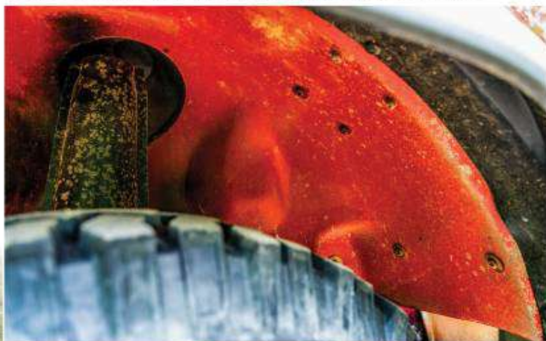
Aluminium inner wings. A closer look reveals axles are all original
