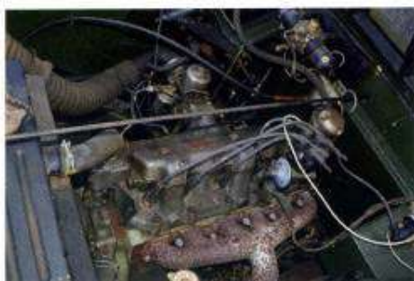
Rover 2.6lt 6-cyl engine.
