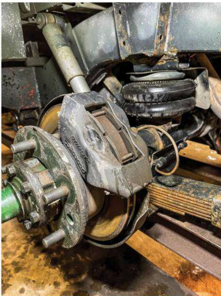
Height-adjustable air springs fitted to mitigate a large increase in vehicle weight
