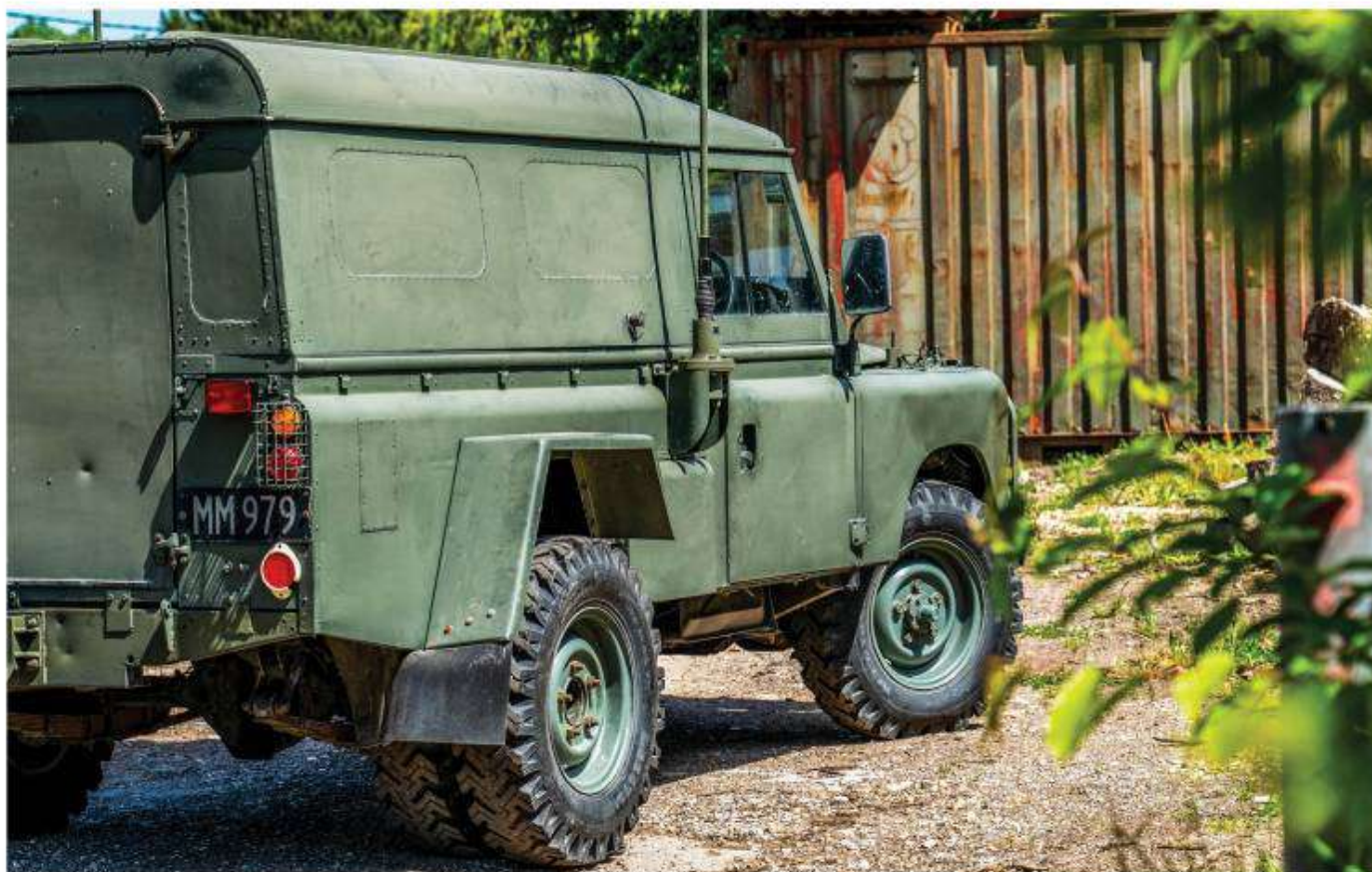
Dual rear wheels fitted to help cope with the weight of electronic warfare equipment – they also give the vehicle an aggressively purposeful look from the rear
