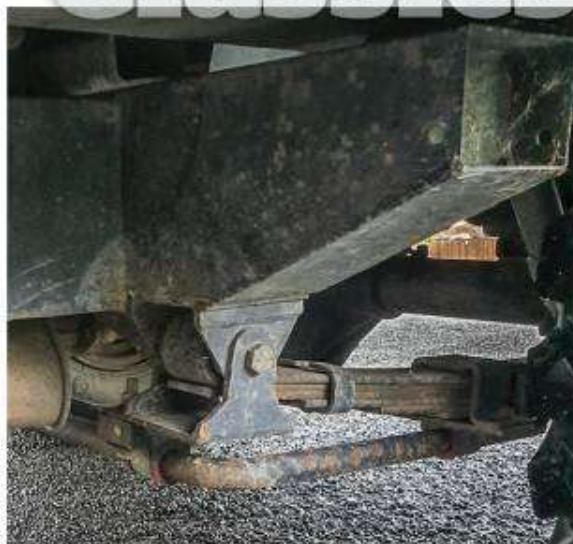
Anti-roll bars attend to some wayward handling characteristics
