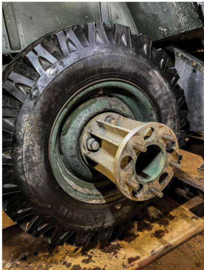
Neat cotton-reel spacer allows fitment of additional rear wheels
