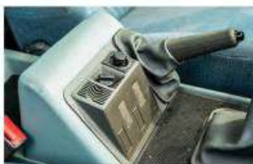
Jay 5 has a prototype five-door window switch panel (above) and white paint added in period to transfer 'box knob
