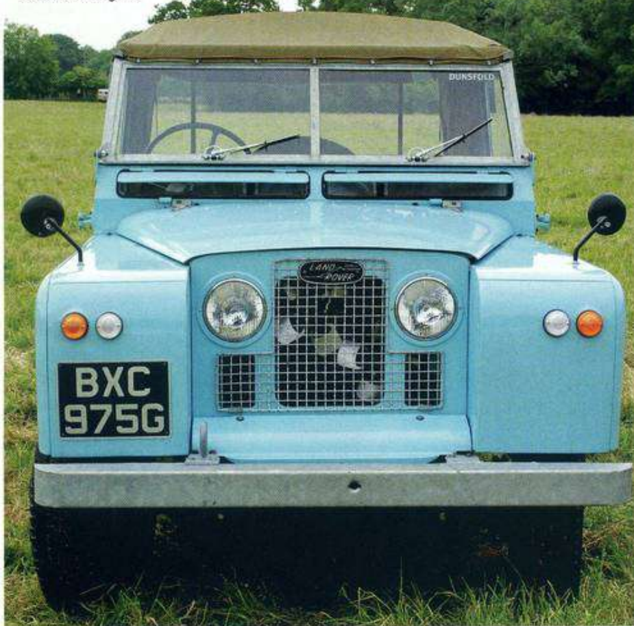
Cooling fan just visible behind grille
