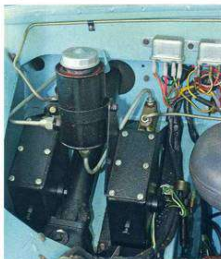
Single line brake system with remote servo
