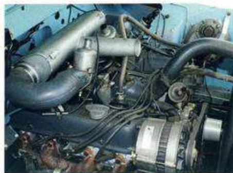
SU carbs, production Range Rover engine had Zenith-Strombergs
