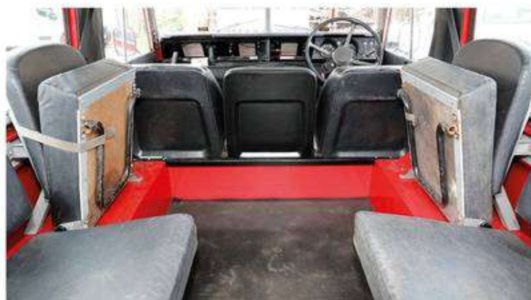
Rear bulkhead removed at the factory
