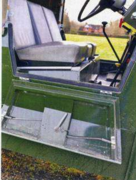
LEFT: Doors are an integral part of the amphib's hull; BELOW: The beautifully-finished and painstaking restoration of the OTAL following a spell in the Dunsfold workshop
