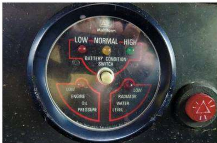
'Multiform' gauge showing battery condition, coolant level and oil pressure
