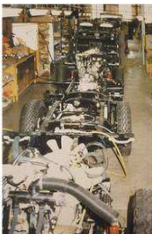
NZ Army 109 V8s being assembled at NZMC plant in Nelson
