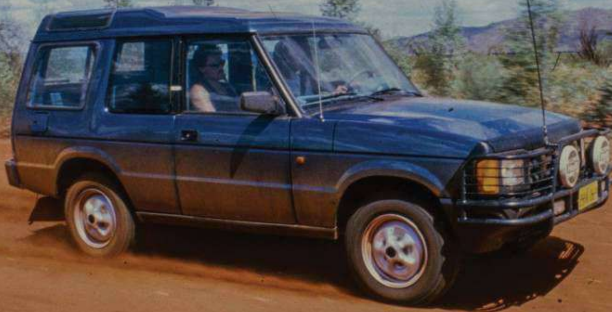
Jay 18 during its extended mileage testing in Australia. Note what appears to be a Range Rover-type decker panel at the base of the windscreen. In fact, the panel line is fake
