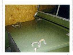
things) and I managed to prise LO9 away from him. It didn't need much doing, as you'd expect, but I rebuilt the gearbox and I upgraded it with a correct pre-pro bonnet, which has 1/8-inch rather than 3/16-inch domed rivets and a slightly different style of ribbing on the underside. Of course, you can't just go out and buy a pre-pro bonnet, but restorer Tom Pickford was having a small batch made by a specialist in alloy so, for a cost of about £1000, I managed to secure one.
