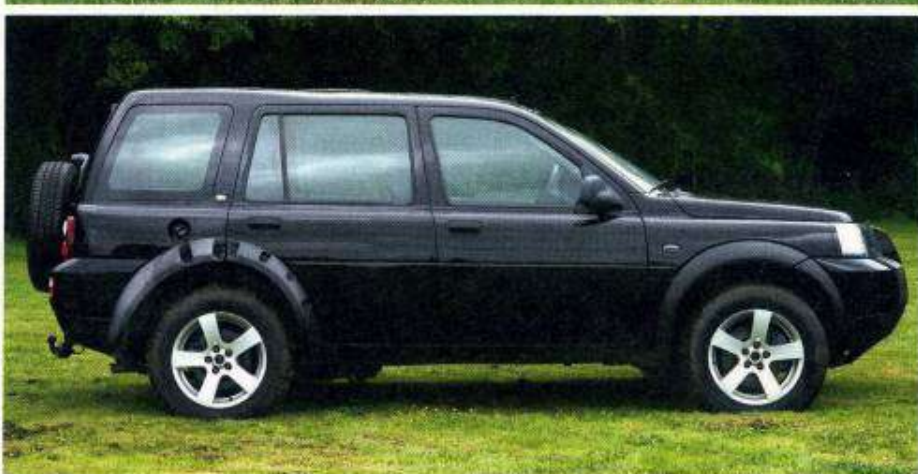
Spot the join? Freelander 2 test mule uses a Freelander 1 bodysell, with stretched rear doors
