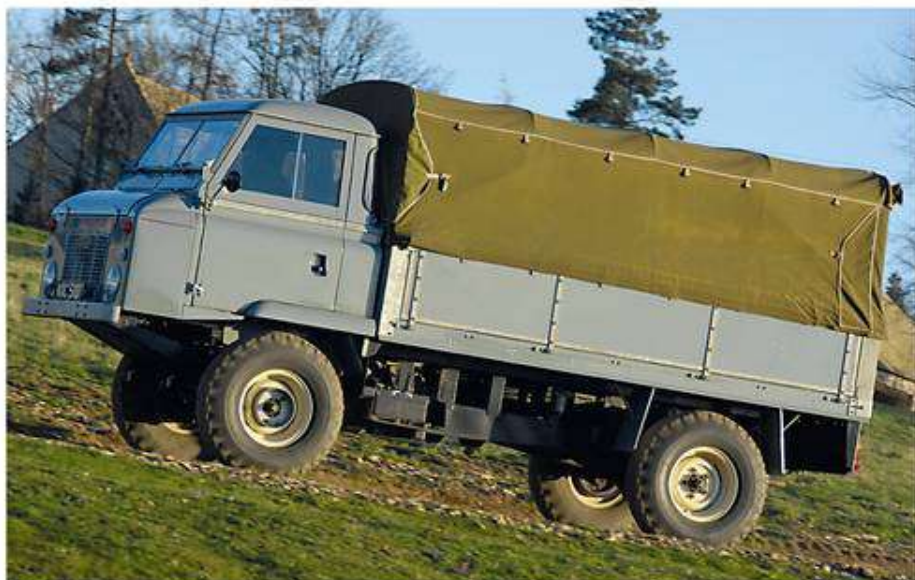
Dunsfold's Series IIB chassis number one is powered – if that's the right word – by a 2.25-litre diesel
