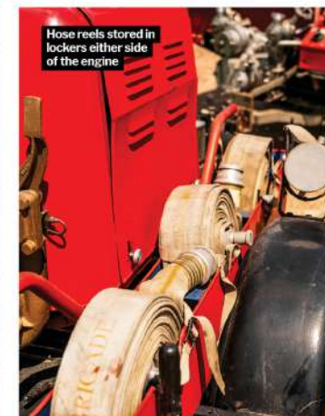
Sigmund pump trailer powered by Morris 8hp engine probably dates from the early 1940s
