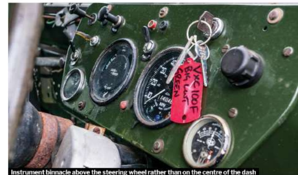
Instrument binnacle above the steering wheel rather than on the centre of the dash
