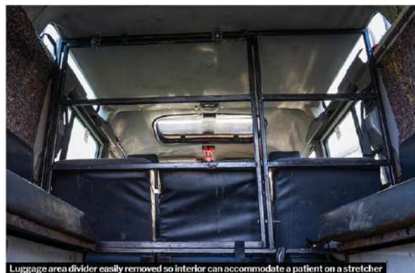
Luggage area divider easily removed so interior can accommodate a patient on a stretcher
