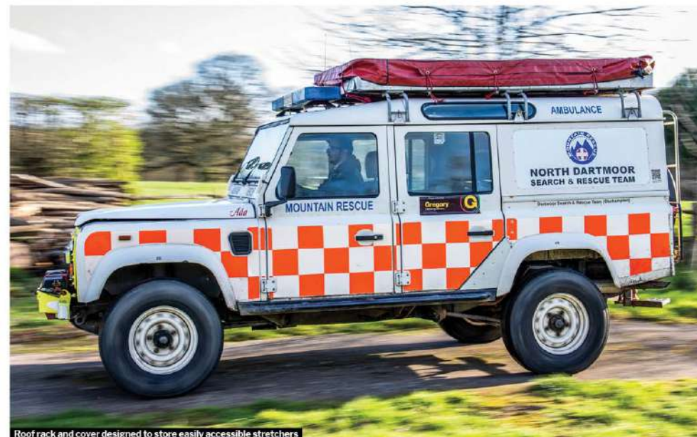
Roof rack and cover designed to store easily accessible stretchers
