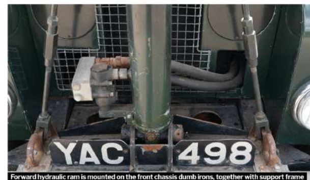
Forward hydraulic ram is mounted on the front chassis dumb irons, together with support frame
