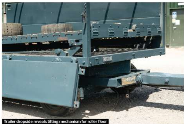
Trailer dropside reveals tilting mechanism for roller floor
